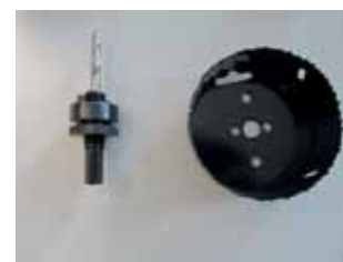
Holesaw, Ø 102 mm, with tool holder for a driller
